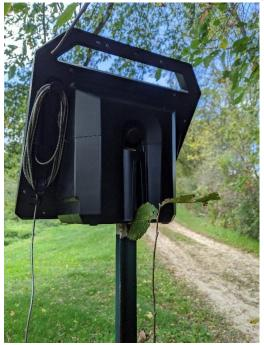
Rotate the unit so that it is facing the direction where it will get the most hours of sunlight during the day. Then lower it onto the post until the post is fully inserted in the slot. Gravity will hold the unit on to the post.
