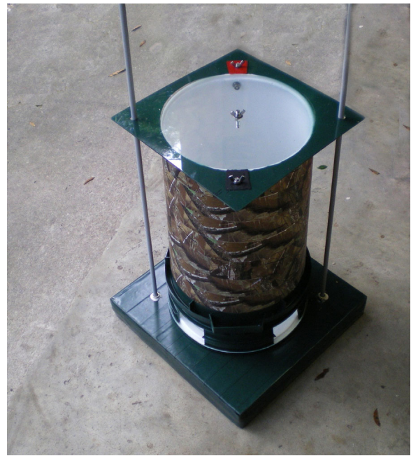
Figure 1. Floating camera trap for small mammals, tested in Florida, USA, during February 2012 to February 2013. The 7-gallon (26.5-L) bucket sits on a base that floats when the tide is high and fiberglass poles keep the trap in place. Lid will be painted white for heat deflection.
