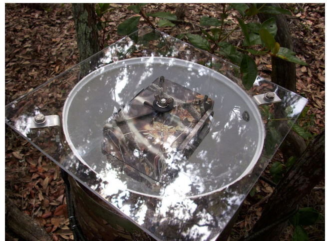
Figure 2. Top view of camera trap showing attachment of camera and lid to body of trap. Note L-brackets on left and right side of photo. Lid is painted white after completion of trap to reflect sunlight and to keep trap and camera cool. Trap was tested in Florida, USA, during February 2012 to February 2013.
